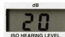
Holding down one of the buttons, the sound pressure is increased or decreased until the button is released. Increments: in the range from -10 dB to 110 dB (refer to max. intensities under Technical Specifications).
