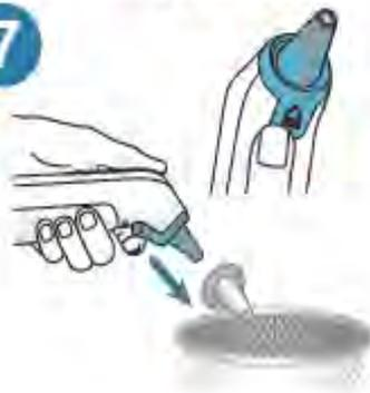
**Remove used probe cover** by pressing Probe Cover Ejector button
