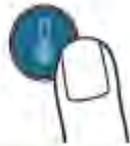
Press and release **MEASURE**
