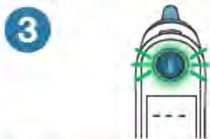
**Wait for the ready indication.** Ring around MEASURE
