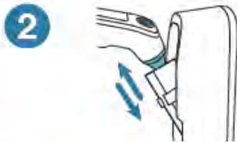
**Attach a new probe cover** by pushing probe tip straight into box, then pulling thermometer out.
